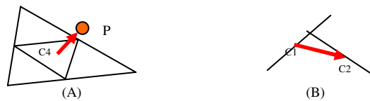
Fig. 3. The red arrow in (A) is the collision normal in the point and triangle collision detection result from figure 1. The red arrow in (B) is the collision normal in the edge and edge collision detection result from figure 2 (A)
