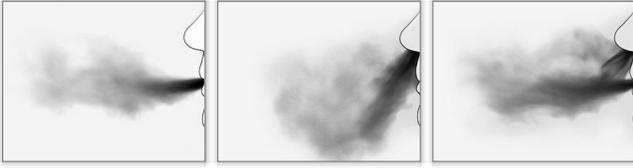
Fig. 4. Recorded turbulent exhale flow from the mouth (left), nose (center), and both nose and mouth simultaneously (right). Through our imaging process, we obtain an accurate illustration of the  $CO_2$  density distribution and flow behavior with minimal background interference.
