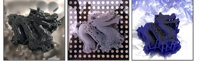
Fig. 9. Volumetric perforation printing process (SLA) illustrating the resin print (left), alcohol wash (center), and 405[nm]-UV cure (right).
