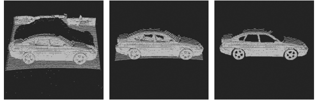
Figure 3. Unmodified Raw Data (left), Auto-Filtered Data (center), Manual Painting-Based Data Elimination (right).
