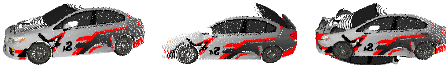
Fig. 5. SAC-IA fails to provide an accurate alignment (right) of the two input point-clouds (left and center) due to the influence of the incorrect correspondence between the trunk and hood
