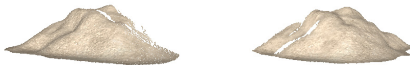
Fig. 2. Illustration of two point-clouds defining a dirt pile surface that lacks unique point-features that would be used for existing key-point selection techniques to generate an estimate alignment
