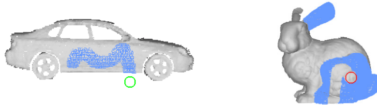
Fig. 4. Brush-based painting tool that selects the data-points within the radius of the brush-selection circle as it is moved across the surface of the scanned object. The unique brush trail left on the surface of the scan illustrates the points selected for alignment (left). The deselection brush allows for points to be removed from the alignment (right).
