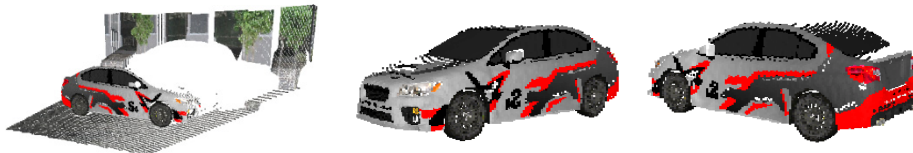
Fig. 1. An example of an individual point-cloud collected with background information present in the time of flight (TOF) scan (left). The front right corner (left) and the rear left corner (right) contain a correspondence overlap of approximately 60%.
