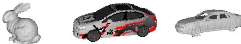
Fig. 8. Alignment results of three individual scan batches: Stanford bunny (left), WRX (center), and the Legacy dataset (right). Through the use of the painting-assisted alignment, highly symmetrical scans can be effectively aligned with minimal human intervention.
