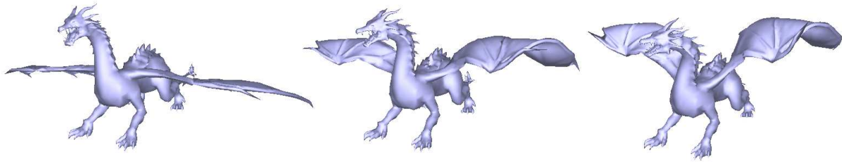
Figure 13: Compound deformations of a dragon raising its wings and rotating its head. The imposed deformations are created from the localized application of four control metaphors. The animated result is displayed left to right.
