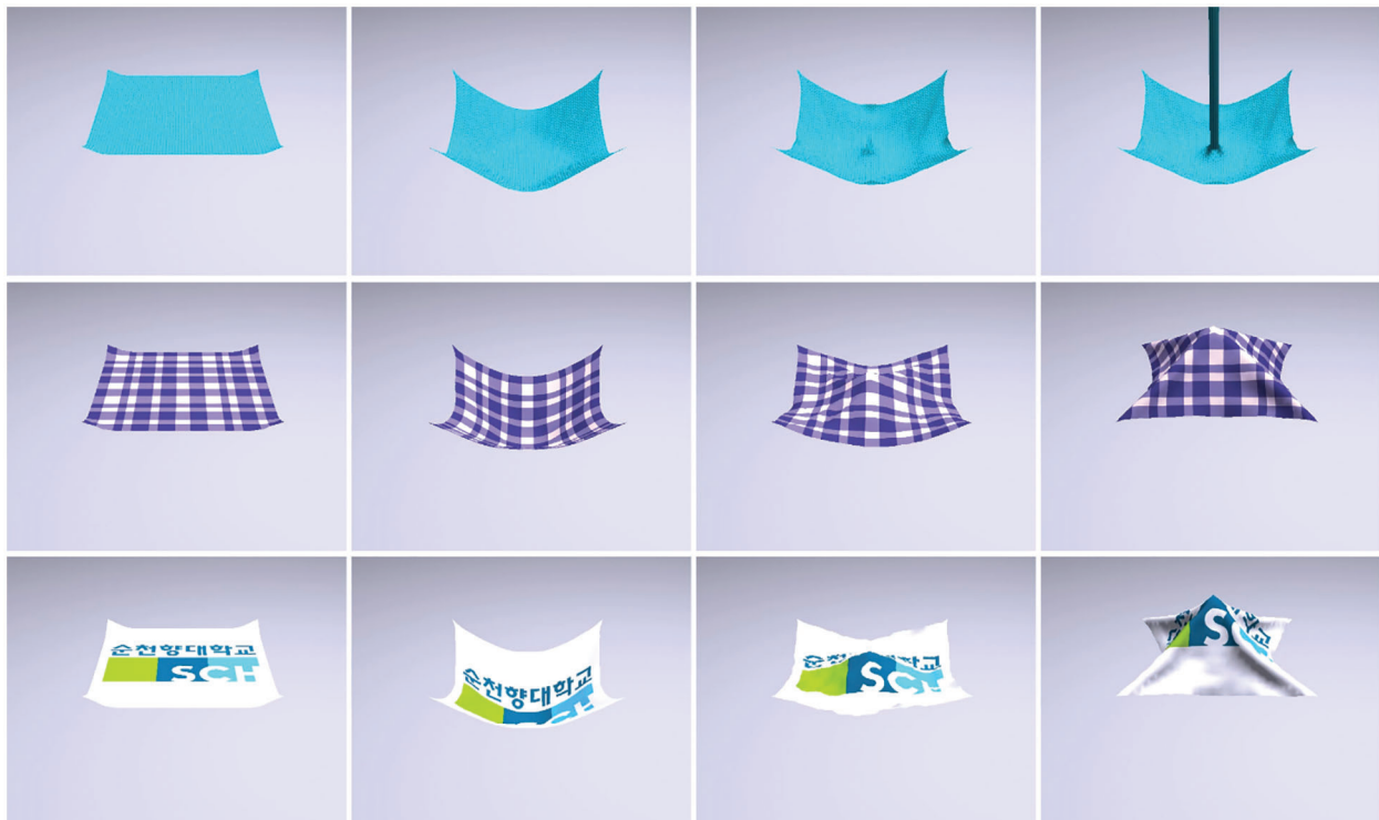
Figure 10: Cloth simulation behavior result when the cloth receives strong force pushing from the bottom of the cloth (time-step = 0.005)
